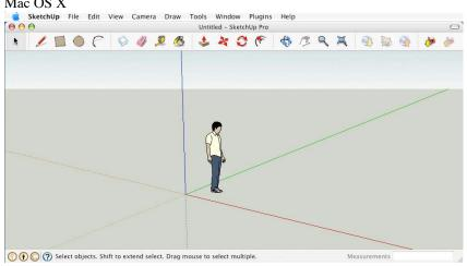
The title bar, at the top of SketchUp, contains the standard window controls (close, minimize, and maximize), the name of the currently opened file, and a title bar collapse/expand button on the right (Mac only). A blank drawing area appears when you start SketchUp and the name of the currently opened file is "Untitled" in the title bar, indicating that you have not yet saved your work.
