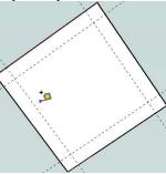
19. Use the Rectangle tool to create the profiles of each chair leg within each corner of the chair bottom. The Rectangle tool will snap to each guide in the corner to make accurate 2" x 2" legs. The following picture shows the resulting four rectangular faces in each corner of the chair bottom.
