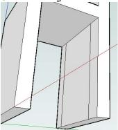
22. Use the Push/Pull tool to remove the area between the back legs.
