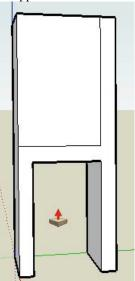
19. Remove the area above the seat and against the back by repeating the process you just used to remove the area below the seat. You're model should now closely resemble a 3D chair (without individual legs).
