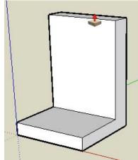
11. Draw an arc across the top of the back starting just below the left side of the back of the chair. Two separate faces will be created at each corner of the top of the chair.
