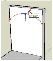
25. Use the Push/Pull tool to remove the two areas at the top of the chair and create a rounded chair back.
