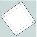
20. Use the Push/Pull tool to create the legs from the four faces created in the previous step. You can use inference to align length of the second through fourth leg to the length of the first leg.
