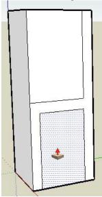
17. Push the rectangular face until it meets the back of the model. The tool tip should say 'on face' when the cursor has met the back face of the model.
