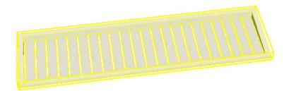
The following image shows the shelf component being edited. Notice that it has a dashed bounding box to indicate you are in the component's context. In this case, a subcomponent, one of the slats in the shelf, has been selected. That slat is within the context of the shelf. Also notice that the component's axes are displayed in the lower left-hand corner.
