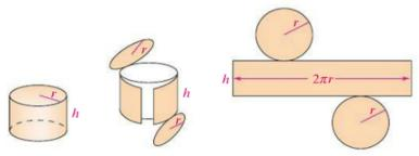
You can use a net of a cylinder to find its surface area.
